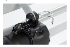
4 | Pin inserted with guard in place.
