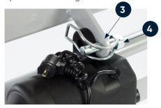
2 | Pin removed and holes aligned.
