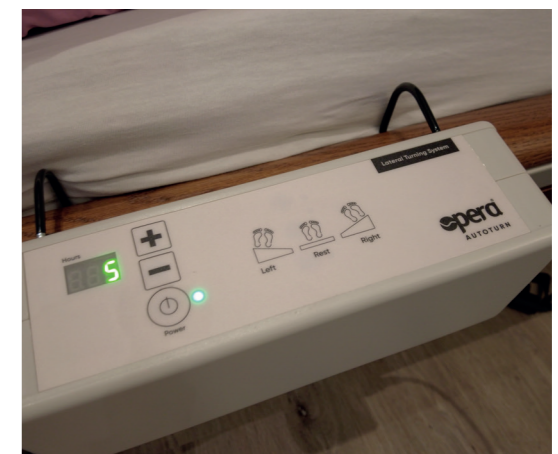
8 Set the timer using the + and - buttons (The number in the timer indicates how many hours the system should run automatically.)
